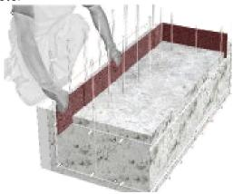
\*In the case of rounded parts and corner constructions, simply bend the AQUAFIN®-CJ7 into the corresponding shape (refer to the image below).
