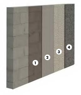
Blocks with binders (e.g. limestone blocks) must have reached an age of at least 6 months before installation of tile and boards (6 months after the production of the block) in order to prevent damage to the tiles, which can be traced back to shrinkage stresses.
