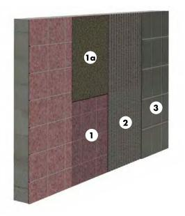
The existing tiled finish must be firm and load bearing. Remove loose areas and level with MGIII cement-based mortar. The substrate must be cleaned and all adhesion inhibiting components, such as lime, grease, dirt, etc., must be removed. Resin repair cracks in the substrate with a reaction resin. Abrading the old tiled finish increases the bond of the primer or scratch coat.
