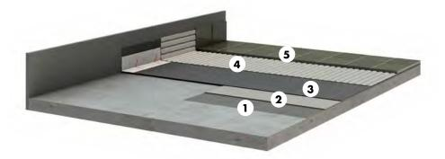
In commercially used wet areas, a particular type of waterproofing is necessary due to the large amounts of water present. The use of bonded waterproof systems (including the bedding mortar for the tiles and boards) protects all building components against moisture.
