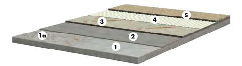
Water soluble paints and adhesive residues must be removed. Lacquers or oil-based paints must be abraded as necessary. Prevent or impede rising damp from the substrate.
