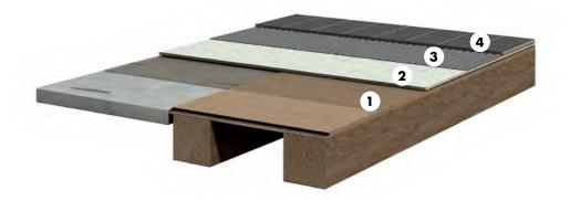
When carrying out building conversions or renovation work, critical substrates are often encountered. They have to be levelled, de-coupled and impact sound transmission reduced before installing tiles. Here the impact sound deadening and de-coupling board STEPBOARD can be used. To reliably prevent height differences, it is recommended that existing cracks in the substrate are adhesively sealed, e.g. ASODUR-K900.
