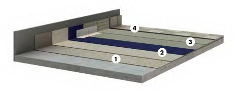
Sauna landscapes have different areas (e.g. dry saunas, steam saunas, showers and other wet rooms) which are subject to different levels of exposure. The waterproofing and installation systems must therefore be adapted to the respective load range. Due to high levels of exposure to steam in a steam sauna, the waterproofing and installation system must also have a vapour barrier function. This can only be fulfilled by reaction resin systems.
