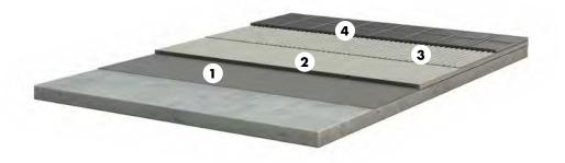
With normal moisture content: CA flow screeds must be abraded, vacuumed and, as with all calcium sulphate substrates, primed with ASO-Unigrund. Heated screeds must be heated in accordance with recognised standards before
