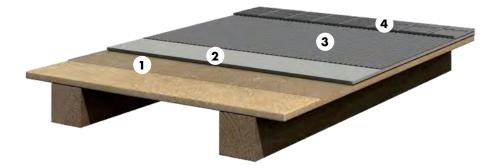
Wood substrates must be clean, dry and load bearing. Chipboard must be laid bonded, screwed and glued. Faulty wood/board substrates must be replaced, loose floor boards must be professionally fixed (e.g. screws, etc.). Seal joints between boards, planks. Please refer to our additional Technical Information No. 10.
