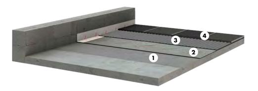
The selection of a suitable system is very important for the sound installation of stone and ceramic on balconies and terraces. Due to different expansion of the materials used, stresses occur
