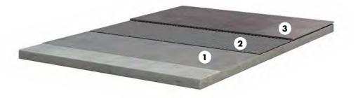
Porcelain stoneware tiles are designated as tiles with water absorption of ≤ 0.5%. This concerns a fully vitrified laying material with an extremely high density. To install porcelain stoneware tiles, polymer modified bedding mortars are needed in order to produce optimum bonding to the very dense surface of the tile. Grouts with accelerated binding are particularly suitable for the grouting of porcelain stoneware tiles.
