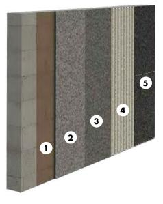
All plasters beneath ceramic tiles or natural stone must be struck off tightly with a straight edge. The surface must remain rough and may not be smoothened or felt boarded. To enable an orderly tile installation, increased requirements for flatness of the plaster should be contractually stipulated.
