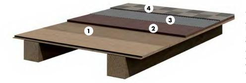
The epoxy resin light screed ASODUR-LE offers a particularly rapid, light and water-free solution for simultaneous levelling of substrates. When installing large format tiles with an edge length over 40 cm and a surface area over 0.18 m<sup>2</sup>, we recommend the following construction design:
