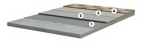
Carry out a moisture test first. The carbide method moisture content may not exceed 2.0 CM% for screed on insulation or separating layers. Heated screeds must be commissioned beforehand. With bonded CT screeds, moisture measurements are not necessary.
