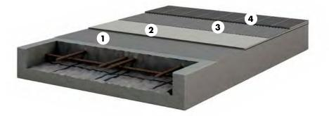
Before waterproofing and tiling concrete substrates it is mandatory to prepare the substrate using shot blasting, high pressure washing or similar techniques in order to remove laitance layers present.
