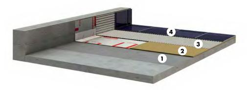
Due to the grouting, tiled and board finishes are not water tight. Therefore, in areas exposed to water, they require waterproofing in order to protect the substrate against moisture.
